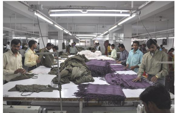
*Energy friendly tube lights have been installed, saving 40% electricity. Overall illumination has improved compared to the old production unit. Also, space is now sufficient for a convenient working environment.*
