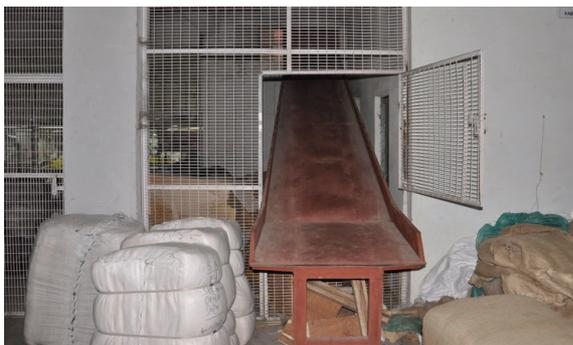
*Slide used for easy transportation of heavy bags with fabric. One end of the slide is at street level where the bags are unloaded when they arrive at the factory, the other is in the cutting department where fabric is processed. At the old unit workers used to carry the heavy bags on their backs.*
